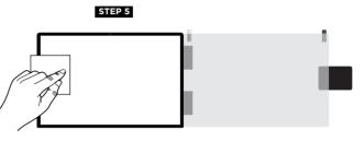
Now unfold the screen protector to one side and clean the device screen. Be patient to remove all dust particles from the screen, use dust removers as needed.
