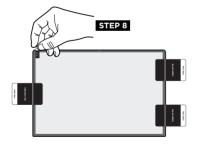
Repeat the above step to clear all air pockets and bubbles. Release the alignment from the side of the device. Hold the screen with one hand and peel off the top layer by pulling tab 2 (surface side).
