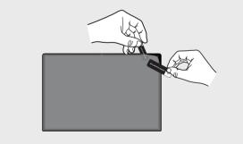
If you notice any dust particles trapped on the screen, stick a dust remover tab on the screen protector, gently lift the screen protector and remove the dust using a second dust remover tab. Repeat **step 9** to complete the application.
