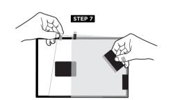
Apply the screen protector holding the alignment tab towards the device. Gently apply pressure with the squeegee to clear any air pockets or bubbles on the screen.
